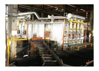
Saudi National Steel produces Deformed Steel Bars from prime quality Billets manufactured in -house. The Billets are inspected and stacked according to cast numbers. Pre-sized Billets are charged to a pusher-type, temperature-controlled Re-heating Furnace.
